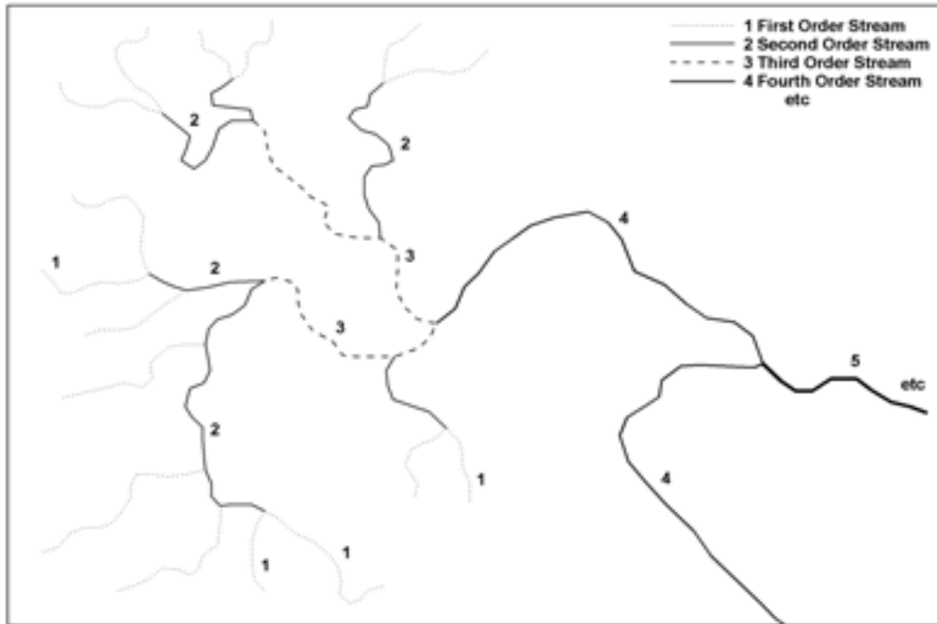
Figure 2: Diagrammatic view of stream ordering
