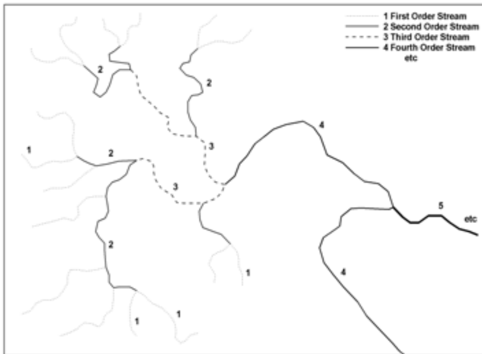
Figure 2: Diagrammatic view of stream ordering
