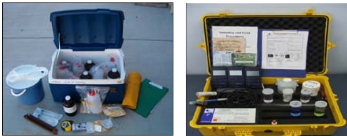
Figure 6. Sampling kits containing all relevant equipment for sample collection (left) and in-situ measurements (right)
