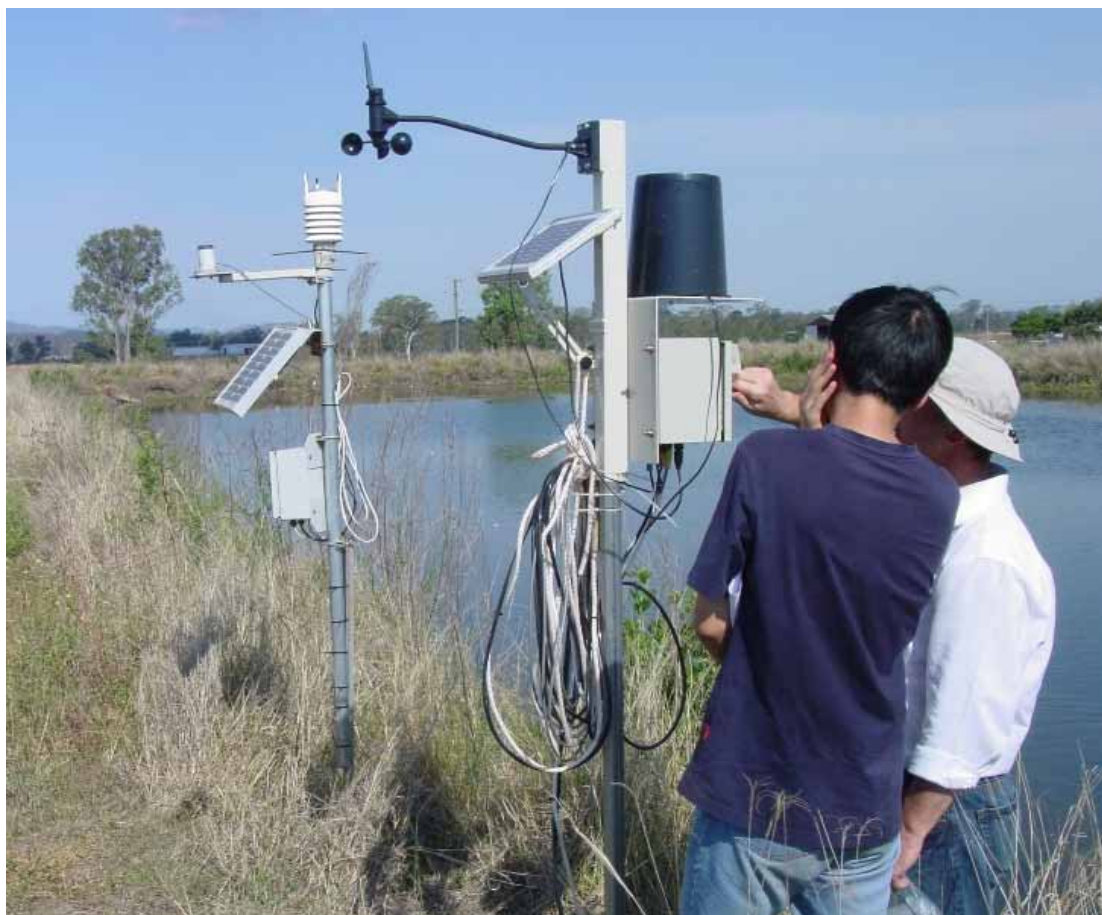
Weather station and seepage meter used to determine water losses from a farm dam
