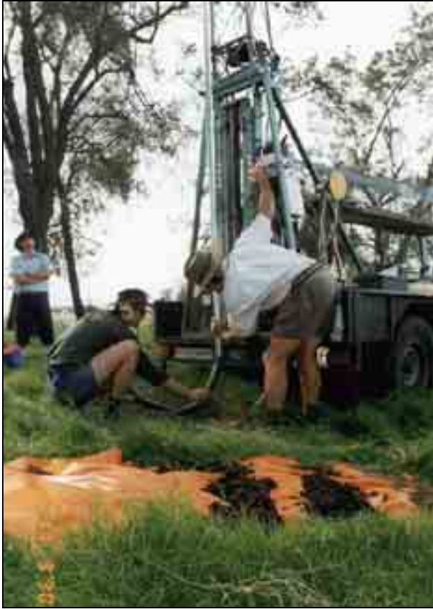
Photo 2. Trailer-mounted vacuum vibro-corer (“Vibrocorer”) sampling rig.
