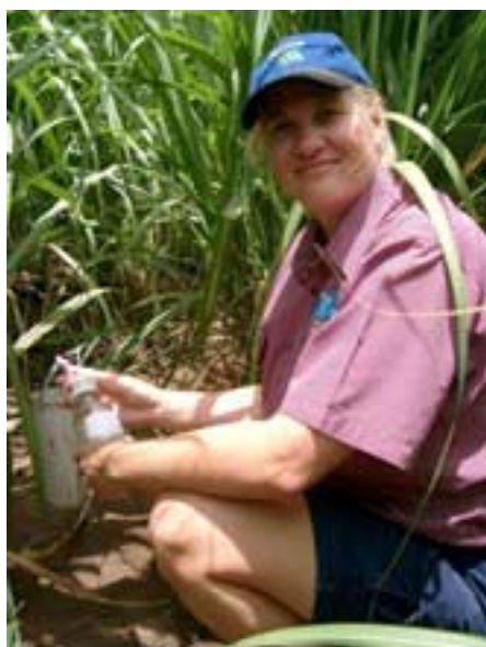
Figure 1 Project officer Jessica Klok with a Schott bottle attached to a suction sampler
